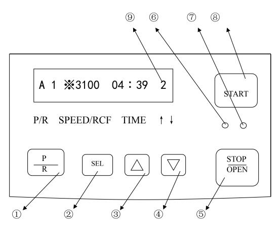
①RCF/RPM; ② Select the program③ Speed/RCF up ④Speed/RCF down ⑤Stop the centrifuge/open the lid ⑥start indicator ⑦stop indicator ⑧start the centrifuge ⑨speed up and down
